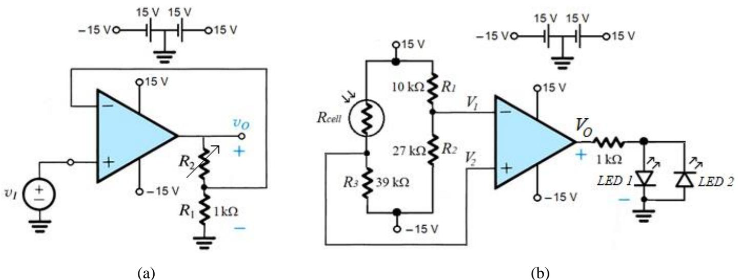
**Figure 6.4** (a) The noninverting amplifier. (b) Comparator to sense light intensity change.
