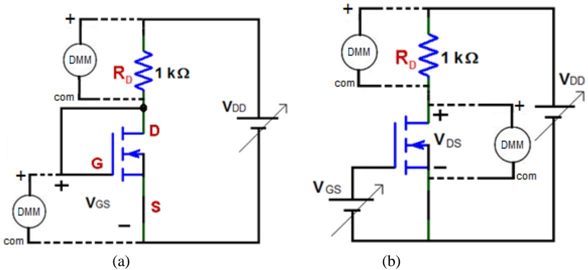
Figure 7.1 Circuit setup for measuring: (a) the threshold voltage, (b) the  $i_D$ - $v_{DS}$  characteristics.
