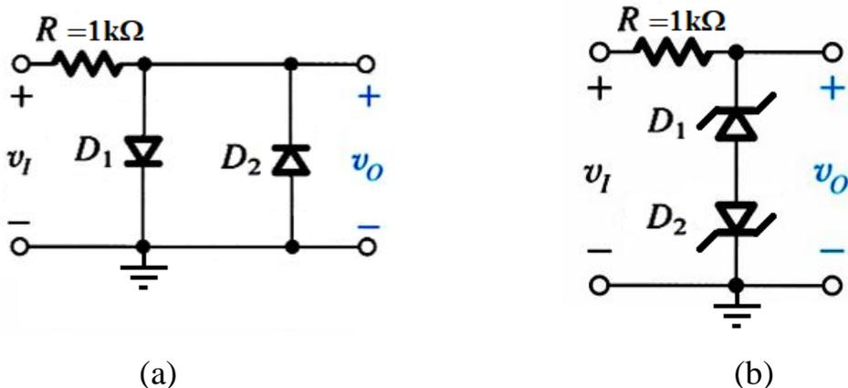
**Figure 3.2** (a) Antiparallel-diode double limiter. (b) Double-anode Zener limiter.
