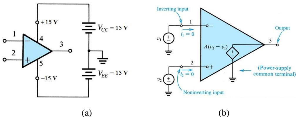
**Figure 6.2** (a) Circuit symbol and (b) equivalent circuit of the ideal op amp [1].
