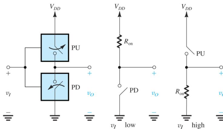
**Figure 8.2** Implementing a logic inverter using two complementary electronic switches [1].
