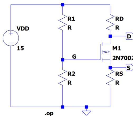
**Figure 9.11** A single supply biasing of a MOSFET amplifier circuit.
