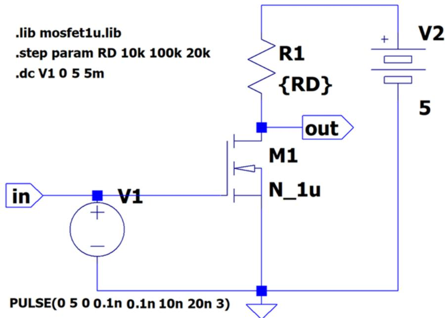
**Figure 8.5** Implementing the CS circuit in LTspice.
