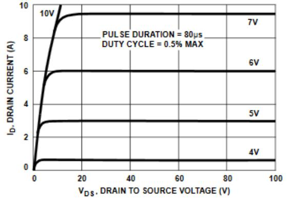
FIGURE 5. OUTPUT CHARACTERISTICS
