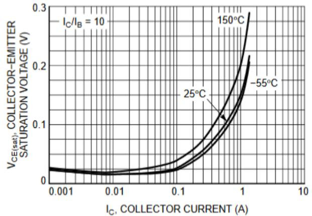
Figure 2. Collector-Emitter Saturation Voltage
