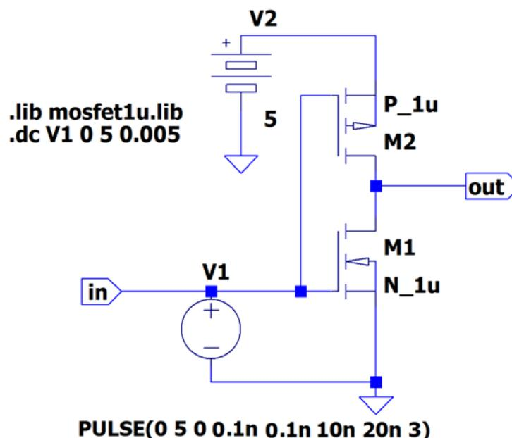
**Figure 8.6** Implementing the CMOS inverter (NOT gate) in LTspice.
