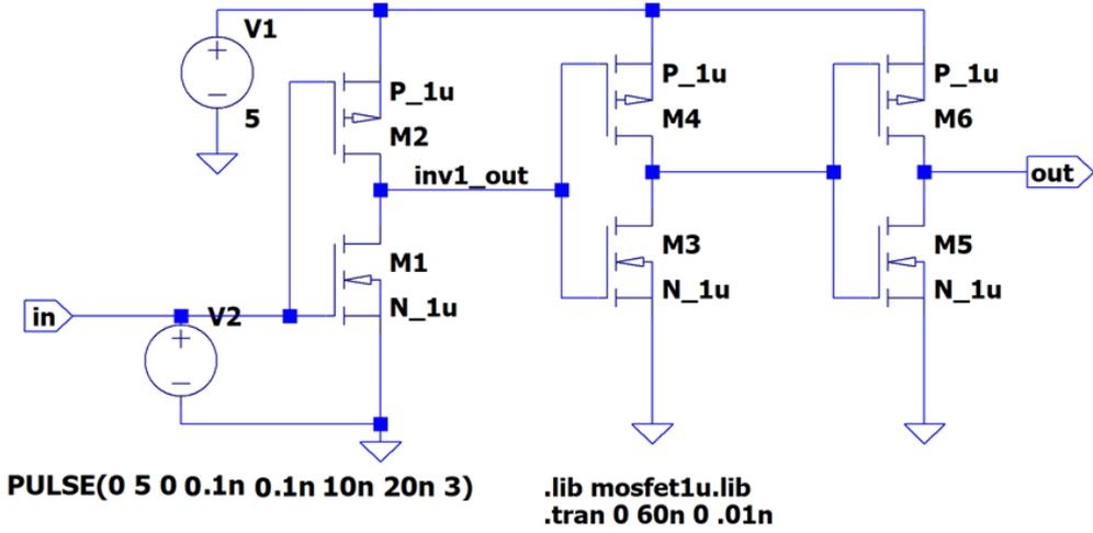
**Figure 8.7** A circuit to explore the effect of cascading on propagation delay.
