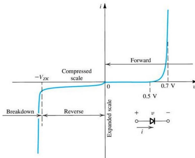
**Figure 2.1** The diode  $i-v$  characteristic curve [1].
