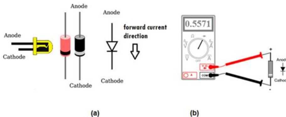
**FIGURE 1.1** (a) Diode shape and symbol. (b) Testing a diode using a DMM.
