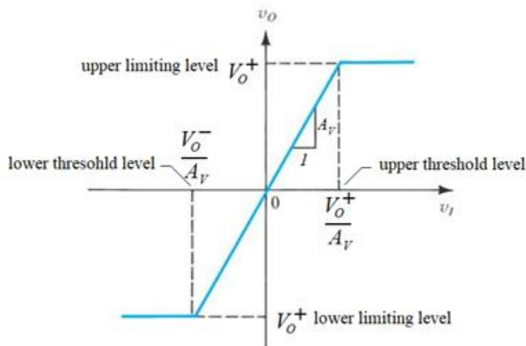
**Figure 3.1** General transfer characteristic for a double limiter circuit.
