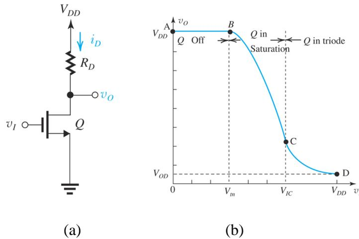
**Figure 8.3** (a) The CS circuit and (b) its transfer characteristic [1].
