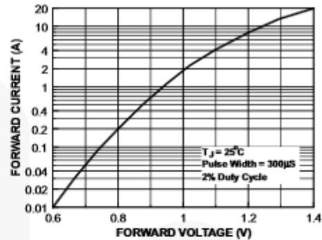
Figure 2. Forward Characteristics
