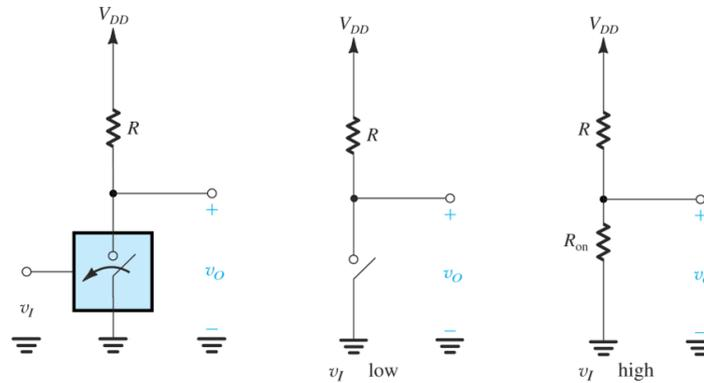
**Figure 8.1** Implementing a logic inverter using a resistor and an electronic switch [1].
