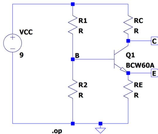
**Figure 9.10** A single supply biasing of a BJT amplifier circuit.
