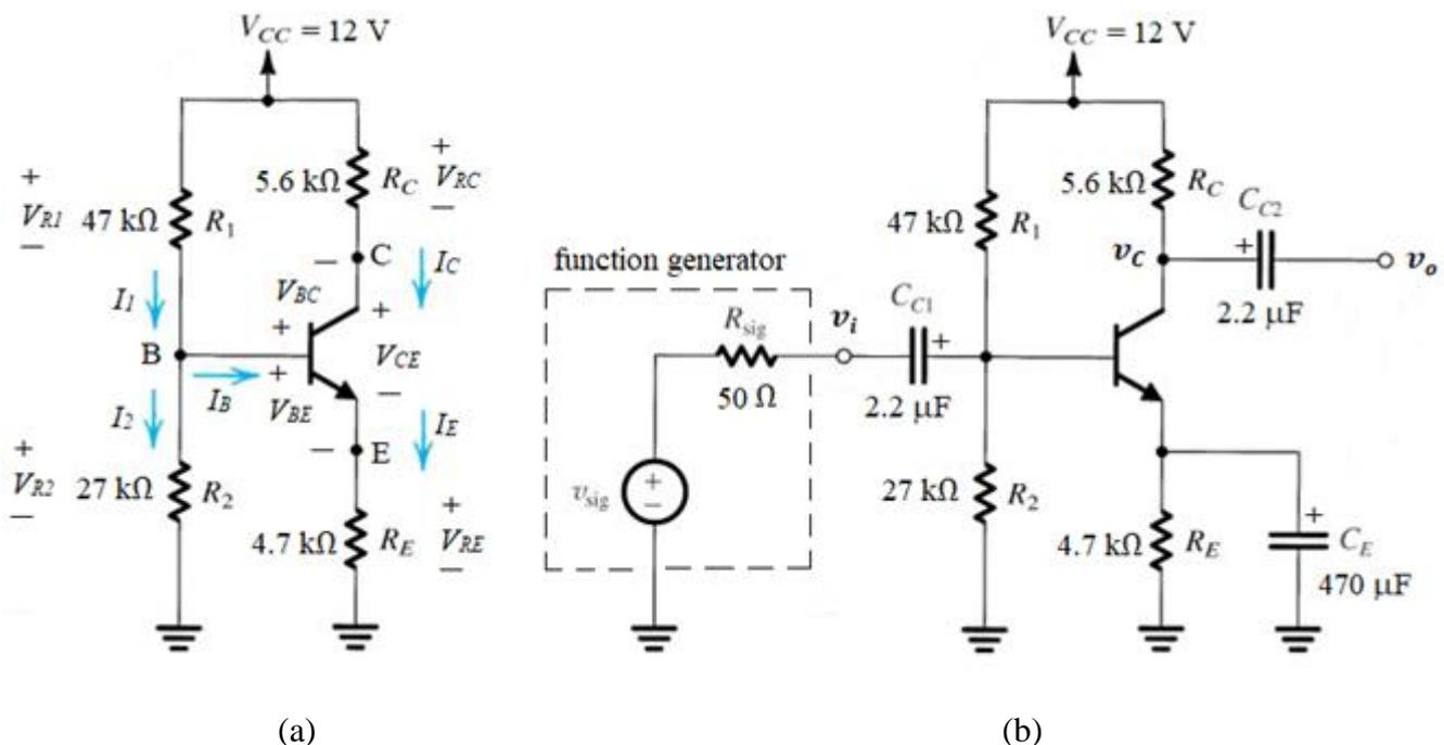
**Figure 10.1** (a) The CE amplifier dc bias circuit. (b) The complete CE amplifier circuit.
