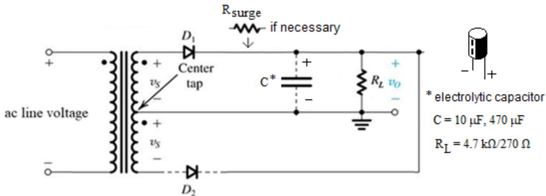
**Figure 4.2** Rectifier circuit which uses a center-tapped transformer.
