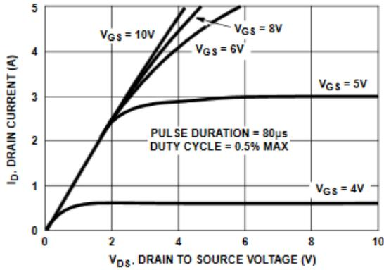
FIGURE 6. SATURATION CHARACTERISTICS
