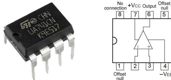
**Figure 6.1** The popular  $\mu\text{A}$  741 op amp IC package and its pin diagram.
