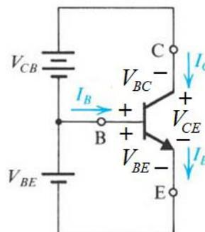
**Figure 9.1** Voltage polarities and current flow for an *npn* transistor.
