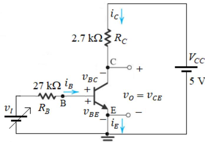
**Figure 9.2** The Common Emitter Circuit.**RESULTS****Table 9.2** Measured Data (Rounded Up to 3 Decimal Places)
