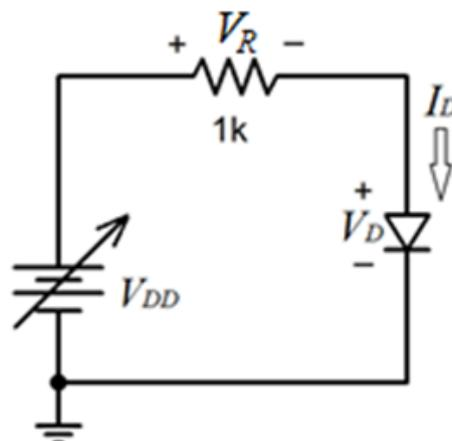
**Figure 2.3** Circuit for measuring the  $i$ - $v$  characteristics.
