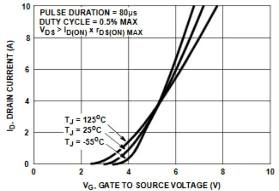
FIGURE 7. TRANSFER CHARACTERISTICS
