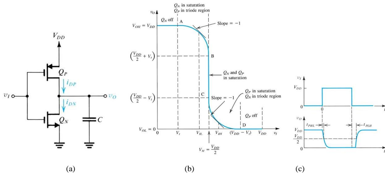
**Figure 8.4** (a) The CMOS inverter, (b) its transfer characteristic, and (c) its dynamic response. [1].
